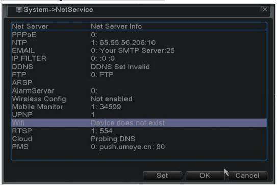
Double click it (or select **Wifi** and press **Set** button) and enable it - tick **Enable** field. You can enable **DHCP** as well.
