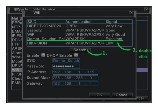
HVR will fill **SSID** field automatically then and you need to put in your wifi password in **Password** field.
